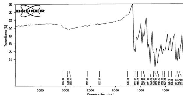
**Fig-3:** the representative FTIR spectra for the Azo aniline compound, **B-III-a**
