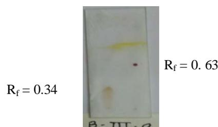
**Fig 1:** The representative TLC for monitoring the reaction of **B-III-a**.
