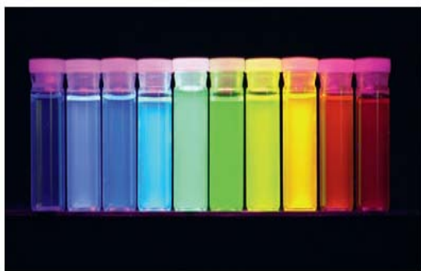
Fig: 10 Semiconductor quantum dots with quantum confinement and size-tunable optical properties. this image shows ten distinguishable emission colors of ZnS-capped cdse quantum dots excited with a near-UV lamp. from left to right (blue to red), the emission maxima are located at 443,473,481,500,518,543,565,610 and 655 nm.
