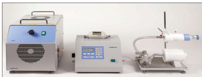
Figure 4: System for testing the dose uniformity of dry-powder inhalers
