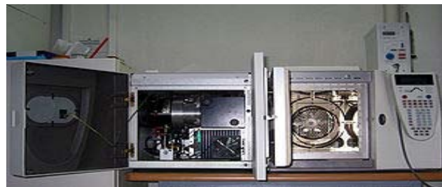
Fig 1: The insides of the GC-MS, with the column of the gas chromatography on the right [6]
