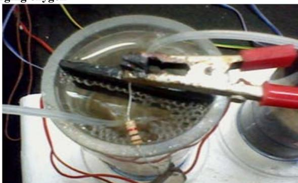
Plate 3: Laboratory set up of SMFC with surface Algae (Sea grass)
