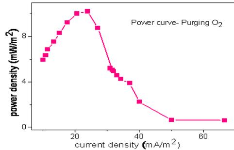
Fig 8: Polarization and power generation curves for SMFC operated with growing algae in sea water
