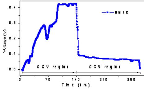
Fig 4: OCV and CCV (at 1000Ω) vs. Time (hrs) for air floated sea water
