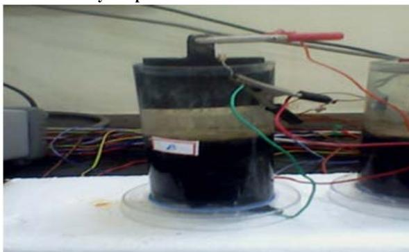
Plate 2: Laboratory set up of SMFC with overlying water with purging oxygen
