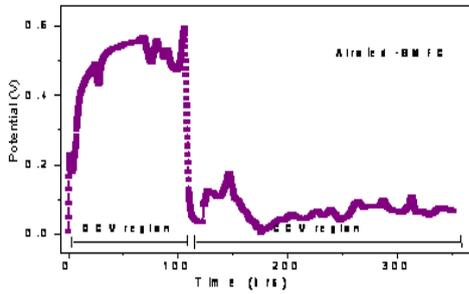
Fig 5: OCV and CCV (at 1000Ω) vs. Time (hrs) for SMFC operated with growing algae in sea water
