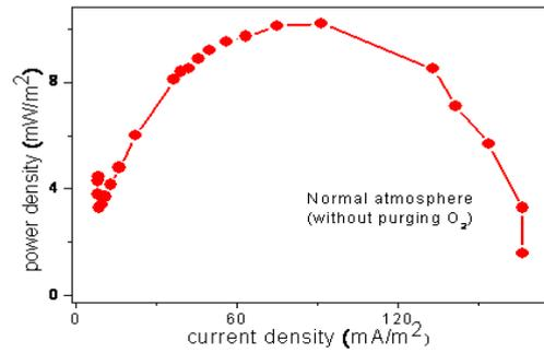
Fig 7: Polarization and power generation curves for SMFC operated with aerated sea water (air purging)
